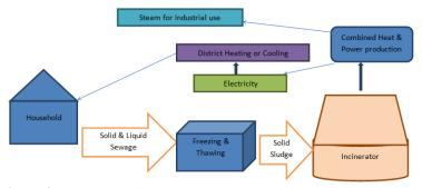
Figure 3. Swedish Model II - Incineration after Freezing and Thawing
