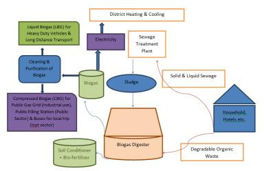
Figure 2. Swedish Model – I: Biogas (through digester)
